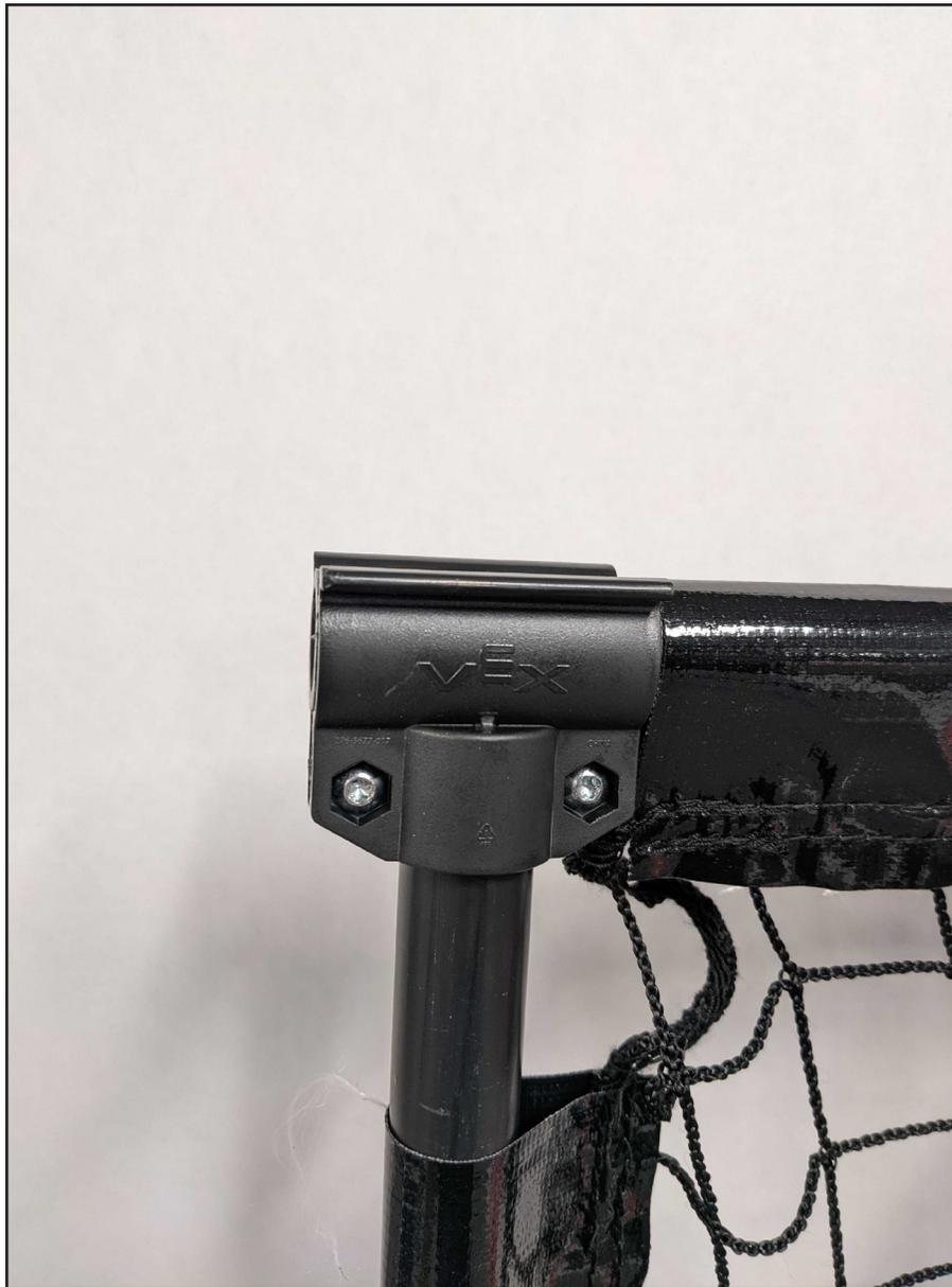
**Problem:** The IQ pieces used to secure the Spin Up Net to the top of a Portable Competition Field Perimeter may not remain attached during gameplay.
