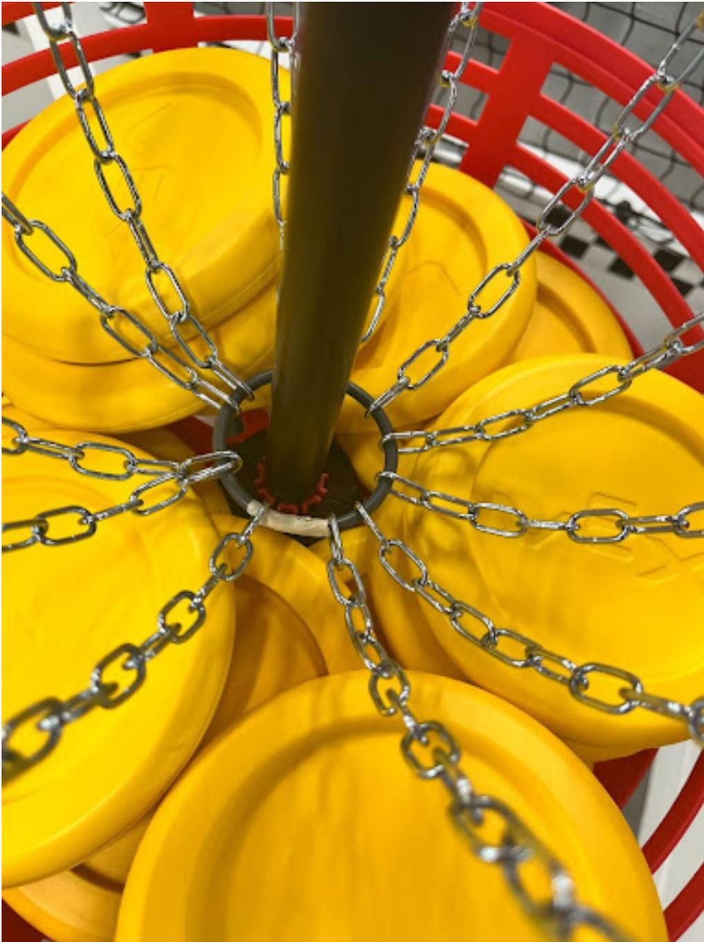
**Problem:** Top connection points could potentially break off of the High Goal, eliminating the ability to connect the chain to the connection point.
