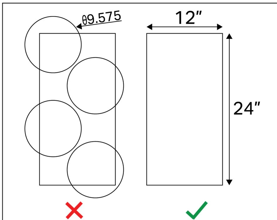
**Figure 23:** Custom plastic parts must fit within a single 12" x 24" sheet of plastic.
