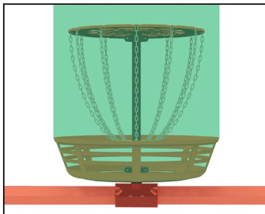
Figure 12: A visual representation of the 3-dimensional volume in which *Discs* are considered *Scored in the High Goal*
