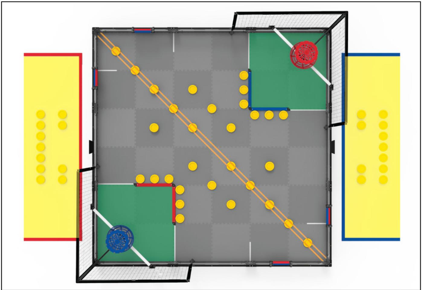
**Figure 3:** Top view of the field with highlighted Alliance Stations (yellow), Low Goals (green), and the Autonomous Line (orange).
